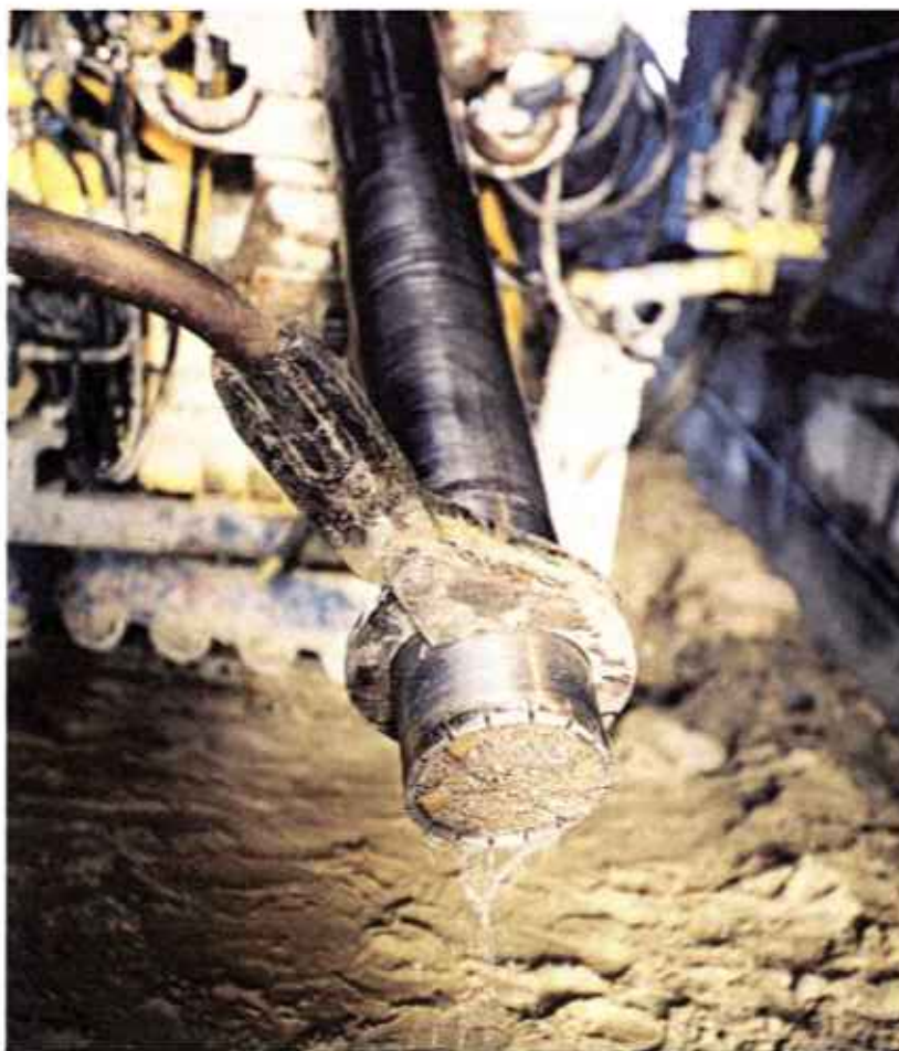
Fig. 3 Break out Core Bit using a Full grip wrench
