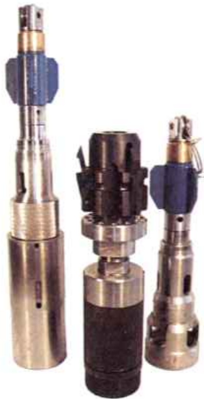
Fig. 13 Geoline – Geobor S Dry hole device, Core barrel head, Overshot
