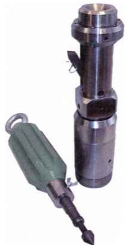
Fig. 14 SK6L Overshot, Core barrel head
