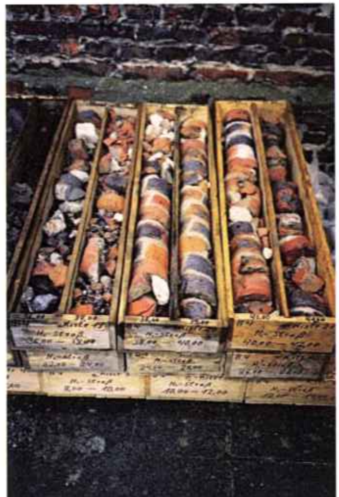
Fig. 5 Core samples from brick stones of an underground shelter
